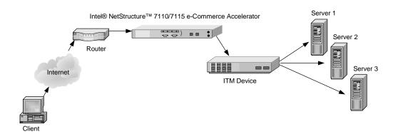
Figure 1-3: 7110/7115 Between Router and ITM Device
